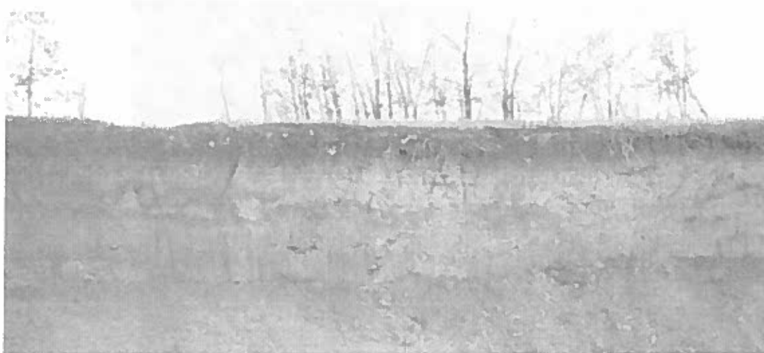
Photo 9: View of operating face that shows faint, thin beds glaciolacustrine silt and clay over massive, blocky brown till.
